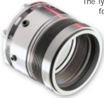
The Type 609 incorporates all of the rugged features of the Type 604, but is intended for those demanding applications where a dependable, high-strength, rotating seal is preferred. A narrow cross-section design enables the Type 609 to fit in the most popular pumps without expensive and time-consuming seal chamber modifications. This makes it the ideal seal for heat transfer, hydrocarbon, and other applications that commonly use pumps with limited seal chamber clearances.
